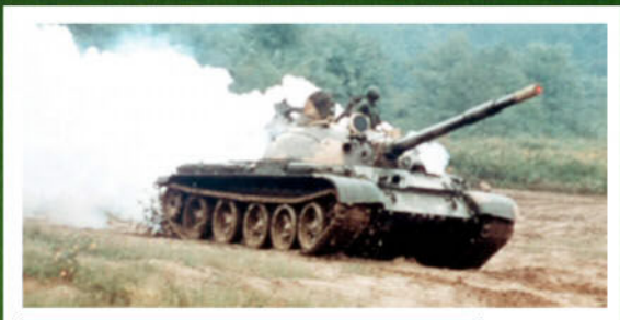
Left: A T-62 main battle tank of the Soviet Red Army lays a smokescreen
